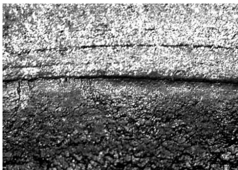
Figure 8 - Macrostructure of a cheek fracture: Transition from the fatigue crack development zone to the brittle fracture zone (50:1)
