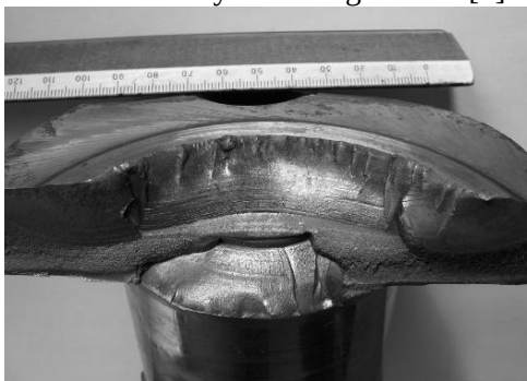
Figure 1 - Form of fatigue failure of the crankshaft along the cheek
