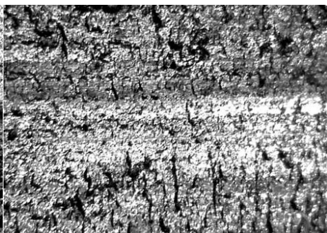
Figure 9 - Macrostructure of a transverse neck fracture: fatigue crack development zone (50:1)
